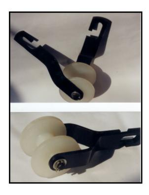
The stringing pulley is designed for stringing small alluminium conductor and overhead telephone lines. Rollers are available in nylon or alluminium. A maximum of 40mm diameter conductor can be used with the stringing pulley. The outside roller diameter is 75mm. Stringing pulleys are manufactured on order only. A lead time of 2 weeks is applicable subject to quantities and roller selection.
